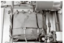
tube sockets, premium F&T electrolytic caps made in Germany, Sozo film/foil replica 'mustard' caps, carbon film and NOS carbon comp resistors, hand-drilled
